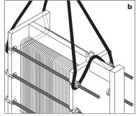
Fastening the round sling to the fixed plate over the top beam
