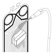
Cleaning of a HE plate with a soft brush under running water
