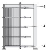
Removing the short tensioning bolts
