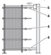
Pushing the loose plate next to the HE plate pack and inserting the tensioning bolts
