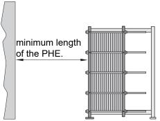
Only for C frames: Recommended spacing from fixed plate
