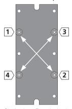
Slackening off tensioning bolts (diagram)
