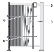
Pushing the loose plate next to the safety stop
