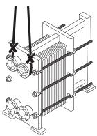
If you fix lifting equipment at the piping connections, these may be bent, may break off or tear off.
