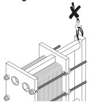
→ Never attach the lifting equipment to the holes drilled in the support.
