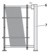
Pushing the loose plate next to the safety stop
