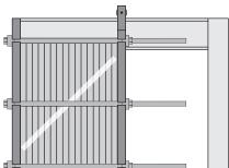
Diagonal strip of paint as an aid for checking the order
