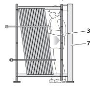
Pushing the loose plate next to the safety stop
