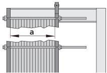
→ Tension the HE plate pack of the PHE within the fixed values a min. < a < a max.
