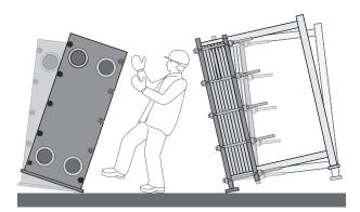
**5.** After putting up the PHE, bolt the PHE down at the place of installation or anchor the PHE at a temporary location before removing the lifting equipment.
