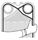
→ Wear protective gloves when working on the PHE and/or with the HE plates.
