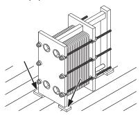
Anchoring a PHE on the floor
