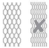
Lateral honeycomb pattern of correctly installed HE plates
