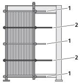
Longer pre-tensioning bolts (from five pairs of tensioning bolts)
