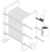
Greasing the tensioning bolt nuts
