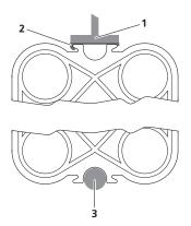
Variant 2: Top beam (1) with special suspension rail (2)
