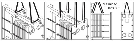
Attach round slings to the shackle holes in the fixed plate and pressure plate.
