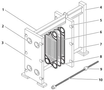
Components of a gasketed PHE
