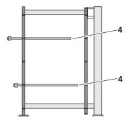
Leaving tensioning bolts in the PHE as a safeguard
