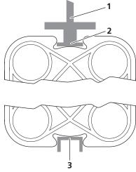
Variant 3: Top beam (1) with special suspension rail B (2)
