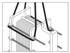
Applying round slings laterally around the top outside pairs of tensioning nuts
