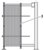
Pushing the loose plate next to the HE plate pack and inserting the tensioning bolts
