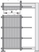
Measuring the tensioning dimension between fixed and loose plate
