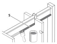
Applying grease along the beam
