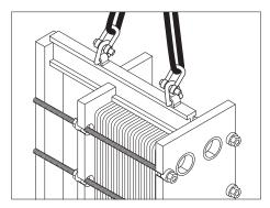
Fastening round slings to shackles fitted in lifting lugs
