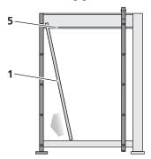
Installing the HE plate into the frame
