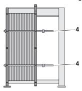
Removing the long tensioning bolts (pre-tensioning bolts)
