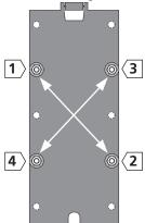
Slackening off tensioning bolts (diagram)
