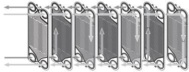
Path of flow media in a single-pass PHE
