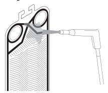
Cleaning away dirt from the HE plate with a high-pressure jet cleaner
